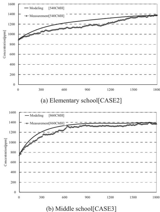
Fig. 6. Comparison of the CO<sub>2</sub> variations between the modeling and the experimental results.
