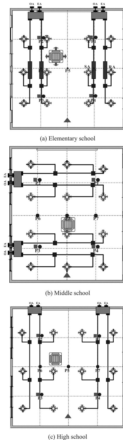
Fig. 2 Installation overview of the air conditioning system, the ventilation system, and the measurement sensors
