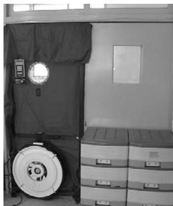
Fig. 1. Photograph of the experimental setup for the measurement of pressure difference.
