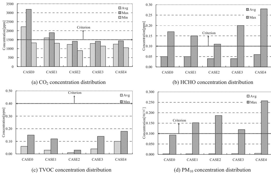
Fig. 3. Measurement results of the indoor air quality of the classroom in the elementary school.
